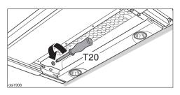
Note for dismantling the cooker hood: Undoing the screws on the left and right inside the housing releases the brackets, allowing the appliance to be removed from the unit.
